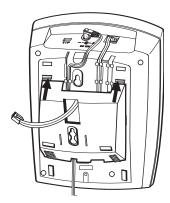
6. Push the tabs on the wide end of the bracket into the lower slots on the bottom of the base.
